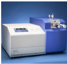
Fischione 1070 Hydrophilization of gold or graphene grids
